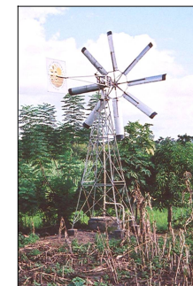
Windmill Pump and Well pipes water to a Reservoir
