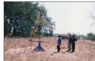
We use a hand-operated Vonder rig so that communities can be involved in drilling wells. They also collect sand for cement.
